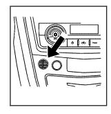
There is an interior temperature sensor located below the climate control system next to the steering wheel.
